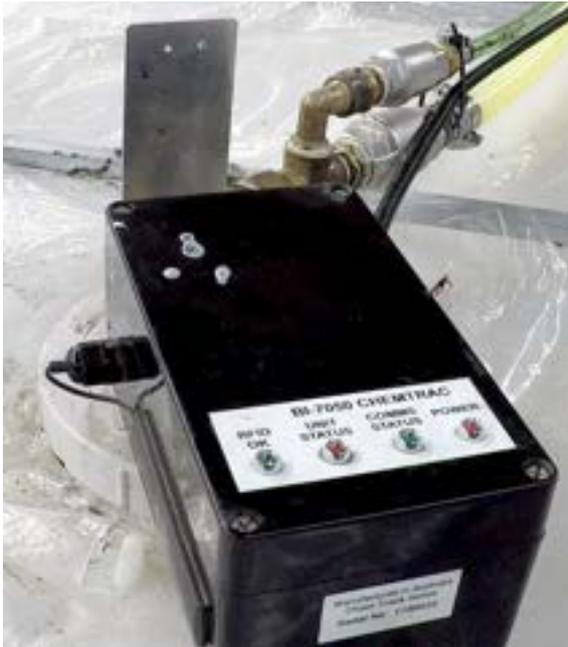
The Bintech auto volume monitoring unit delivers readings of BioClean usage three times a week via the mobile phone network in a graph format pictured below.
